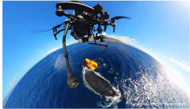
Left: Monitoring crew attached a CATS multi-sensor suction-cup tag to a humpback whale using a long pole. Right: Monitoring crew uses a UAS platform to drop a suction-cup tag on an animal.
