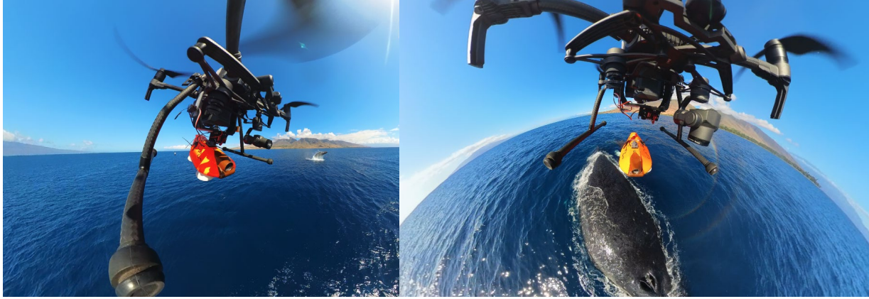
Drone carrying and dropping a suction-cup tag flies over sanctuary waters off Maui as an adult humpback whale breaches in the background (NOAA MMHSRP permit no. 24359)
